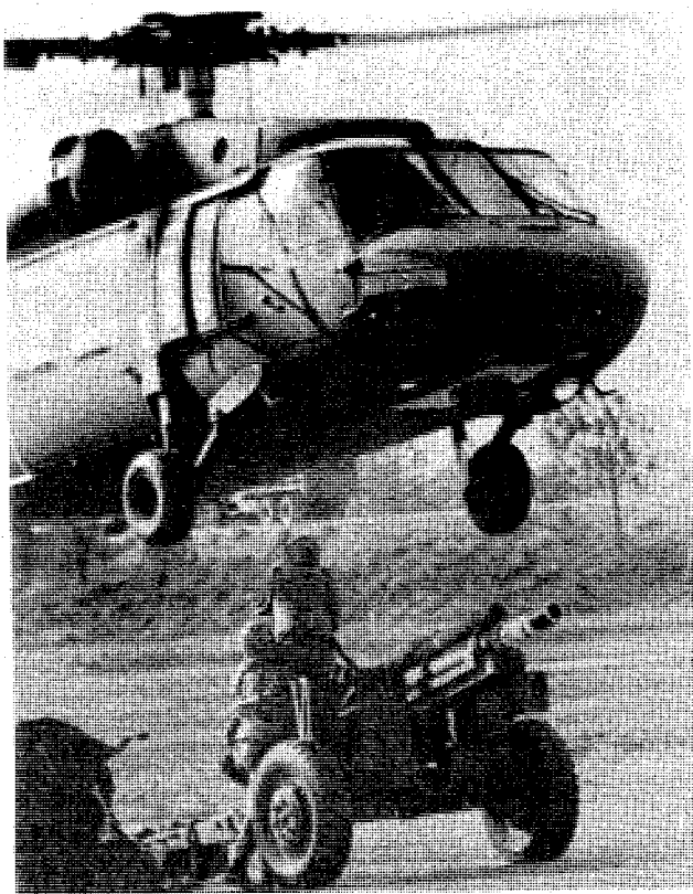
As the hook-up man stands ready on the howitzer, the Black Hawk inches forward so the sling load connection can be made.
