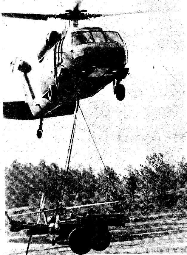
With the gun section crew members aboard the helicopter, it picks up the 1st section's howitzer.
