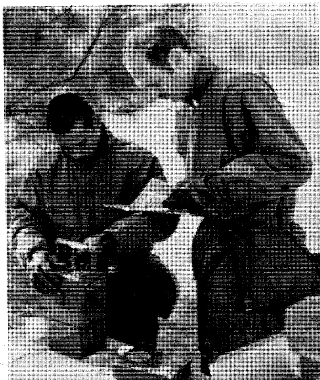
Sp4 Jesus Soto (I) and Pvt. 2 Douglas Russell give the automatic chemical agent alarm a pre-operational check.
