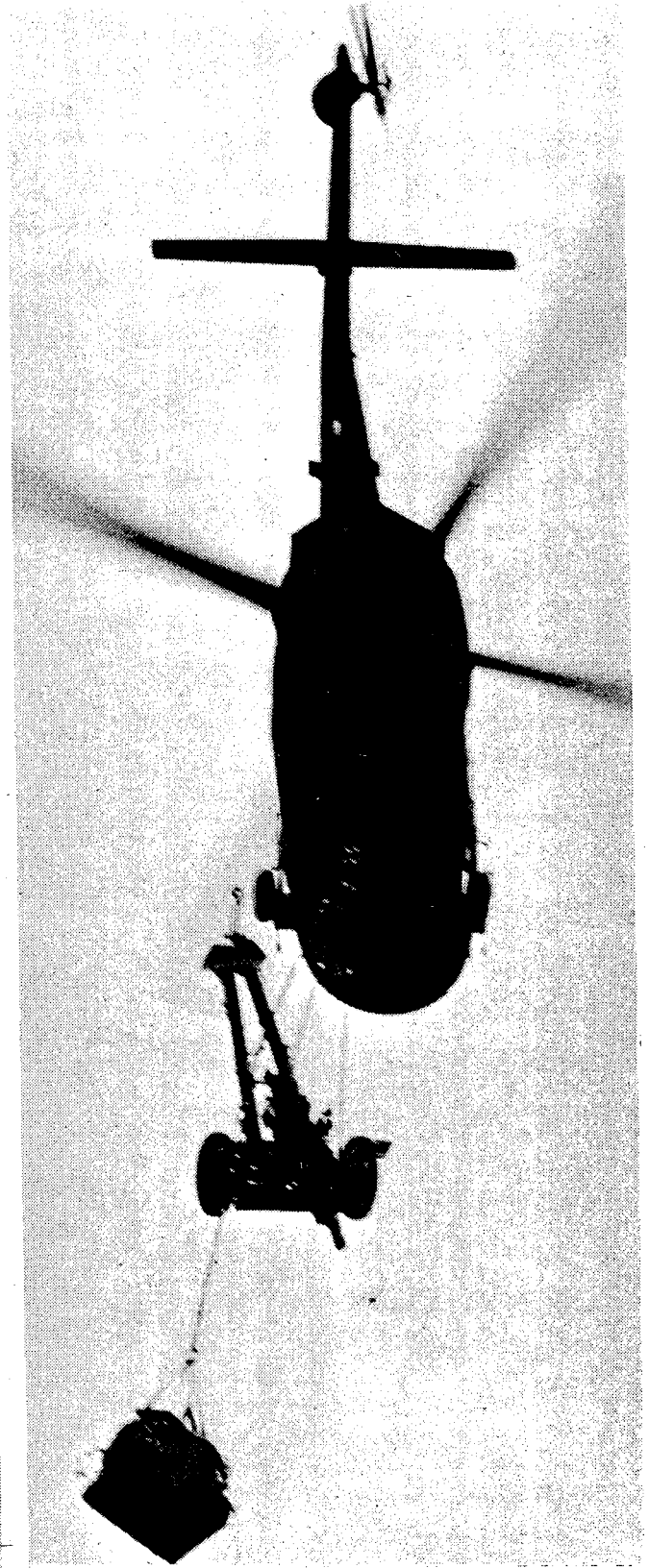
The approximately 5,500-pound combined weight of the howitzer and the loaded ammunition bag presents no problem for the Black Hawk, with its 8,000-pound sling load capability.
