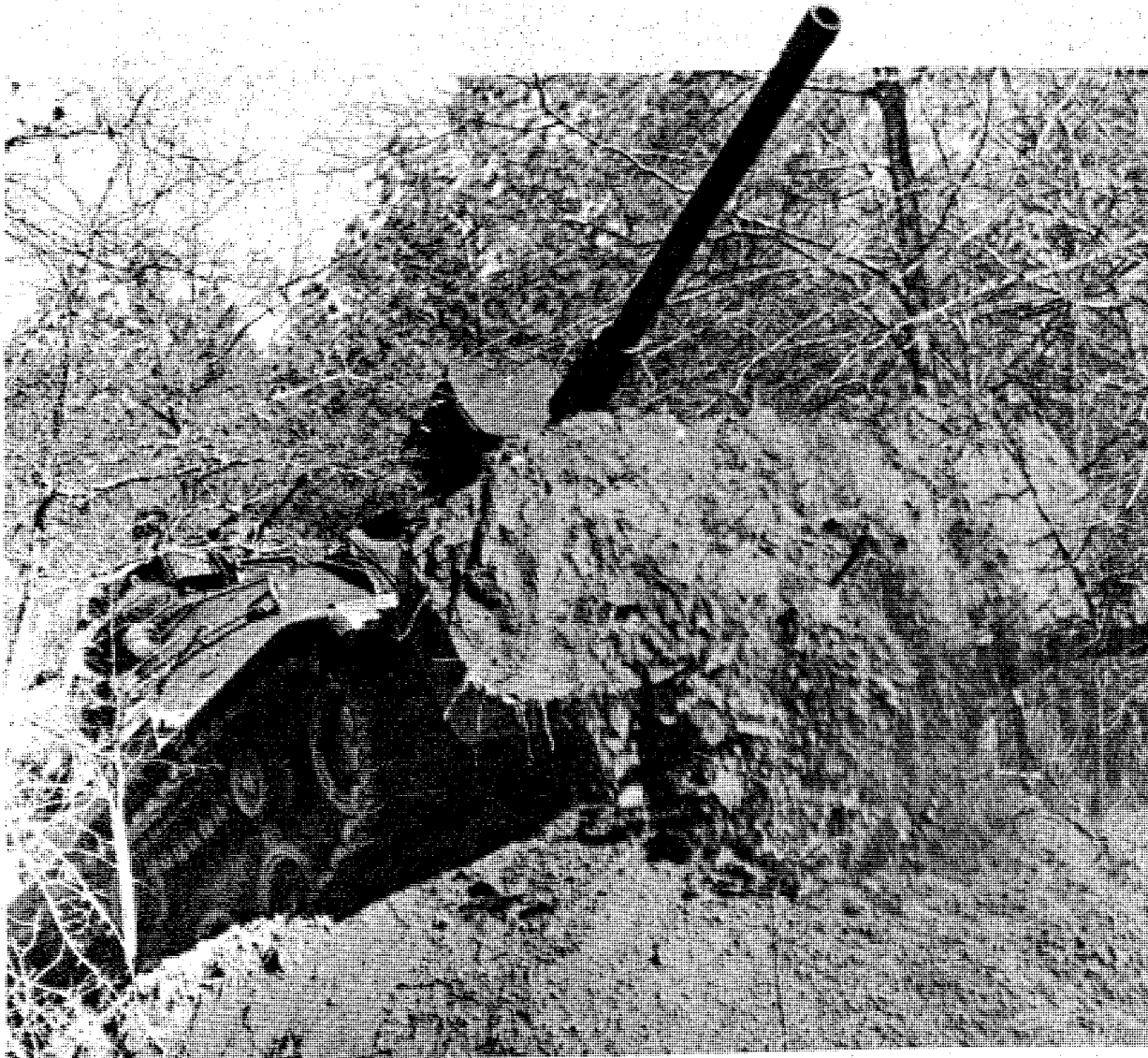
A blade tank pushes through the underbrush to make way for following tanks.
