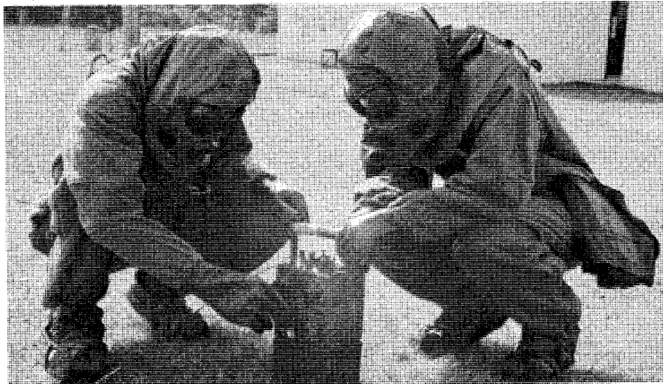
PFC Luis Rodriguez and Pvt. Debra Lovelace employ the automatic chemical agent alarm.
