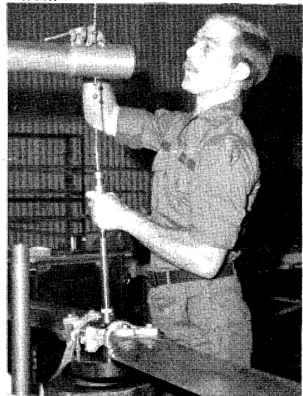
Sp4 David Argo, prop and rotor shop hangs a helicopter tail rotor on a Marvel balance stand in preparation for balancing.
