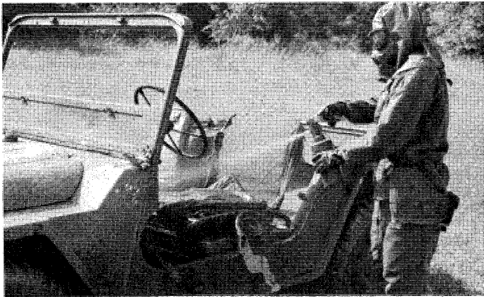
Pvt. Debra Lovelace performs emergency decontamination with decontamination apparatus.
