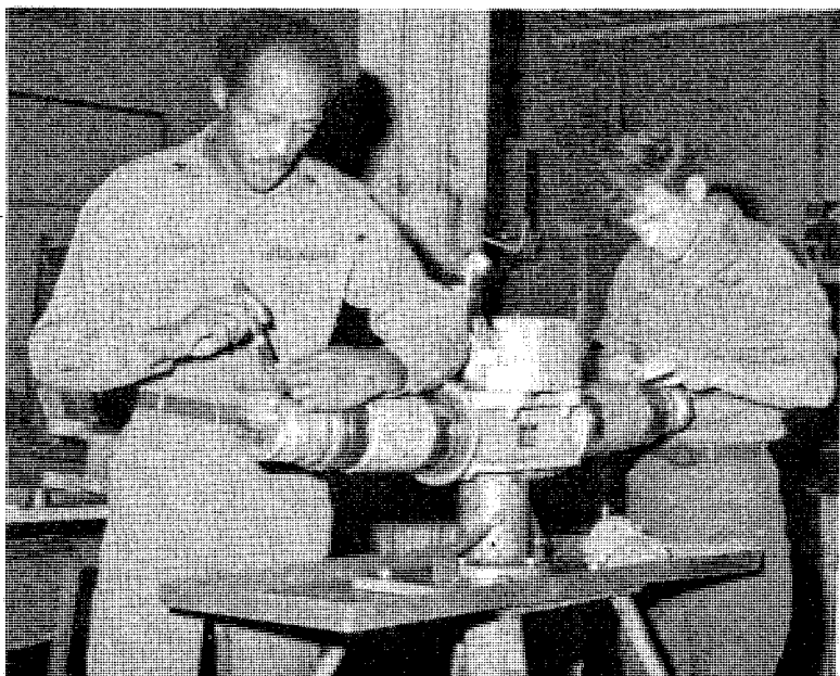
Sgt. Joseph Stokes (I) and Sp4 Dickey Smith, prop and rotor shop, repair a main rotor head.
